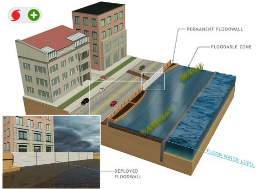
GIF showing deployable floodwall to halt flood advancement
